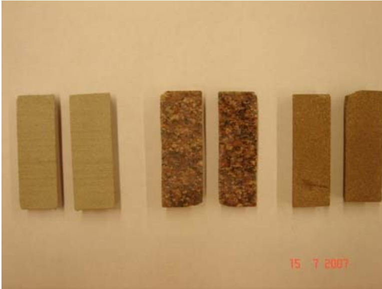
Figure 5-1: Core samples with smooth fracture surfaces. From left to right: sandstone, granite and limestone
