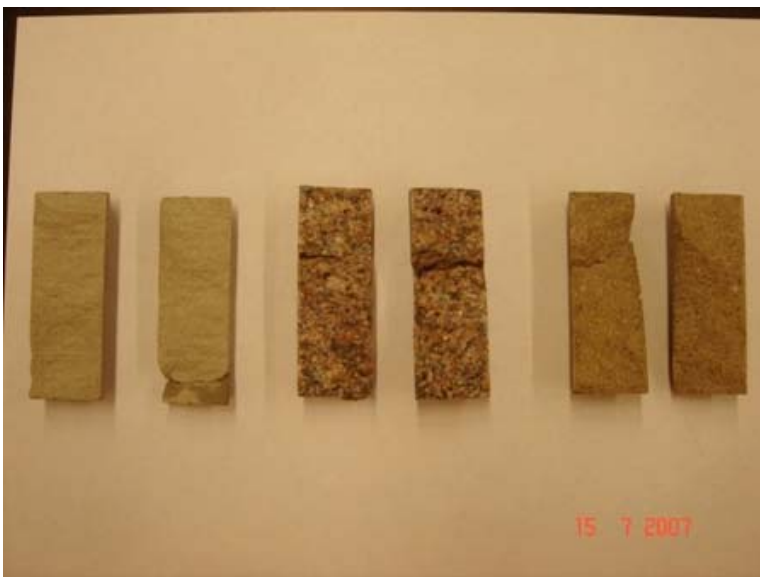
Figure 5-2: Core samples with rough fracture surfaces. From left to right: sandstone, granite and limestone
