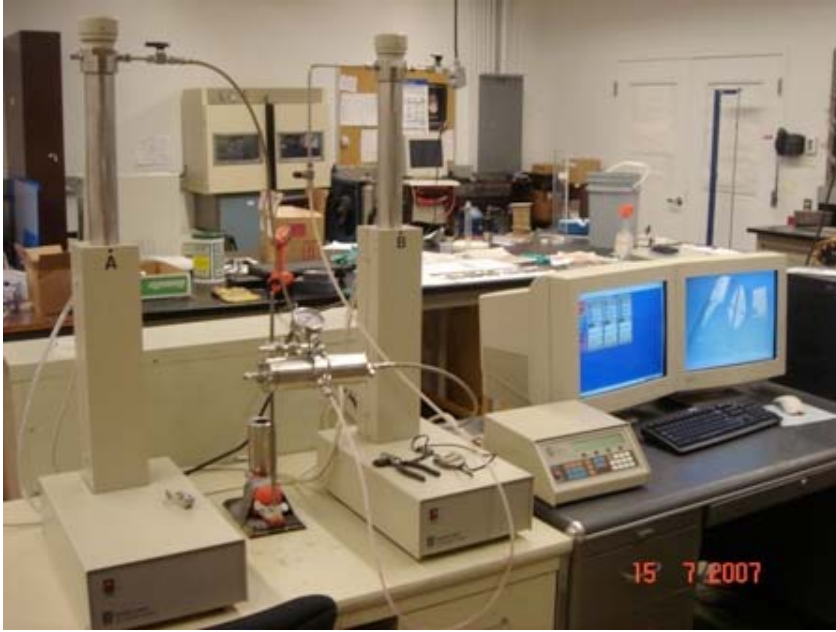
Figure 5-5: The laboratory setup for borehole ballooning experiments
